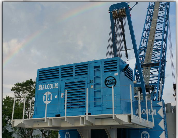
CUSTOM BUILT MODEL 800 POWER UNIT TIER IV FOR MALCOLM, MOUNTED AS A COUNTER WEIGHT ON THE BACK OF A LIEBHERR LR1300 CRANE.
