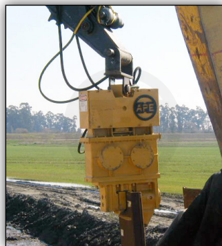
MODEL 20 VIBRO WITH A MODEL 20 CLAMP.
