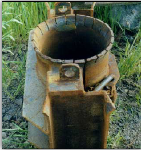
BOX LEAD FIXED PILE GATE.
