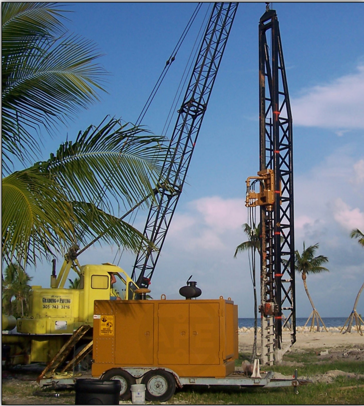
A MODEL 20 DRILL IN A SWINGING LEADER.
