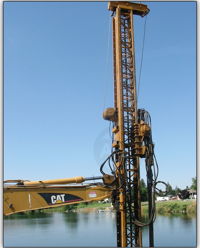
A MODEL 20 DRILL AND AN AD COCKDOWN-THE-HOLE PERCUSSION DRILL.
