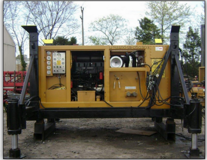
MODEL 350 POWER UNIT MOUNTED IN A HELICOPTER LIFT.
